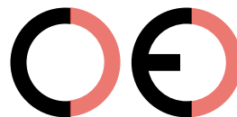
False CE Mark (too far)
