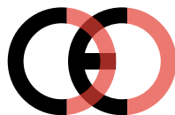
False CE Mark (too close)
